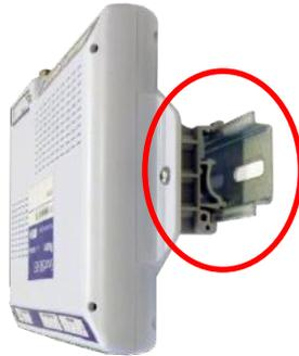
A rack-mount shelf can also be used to install the plenum-mount controllers in a rack-mount cabinet. Simply attach DIN-Rails at the bottom of the shelf.
